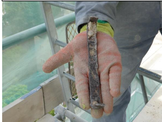
A stonemason holds a corroded iron clamp – the cause of the cracked stones
